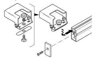
9. Screw extrusion end plates to fence extrusion as illustrated.
